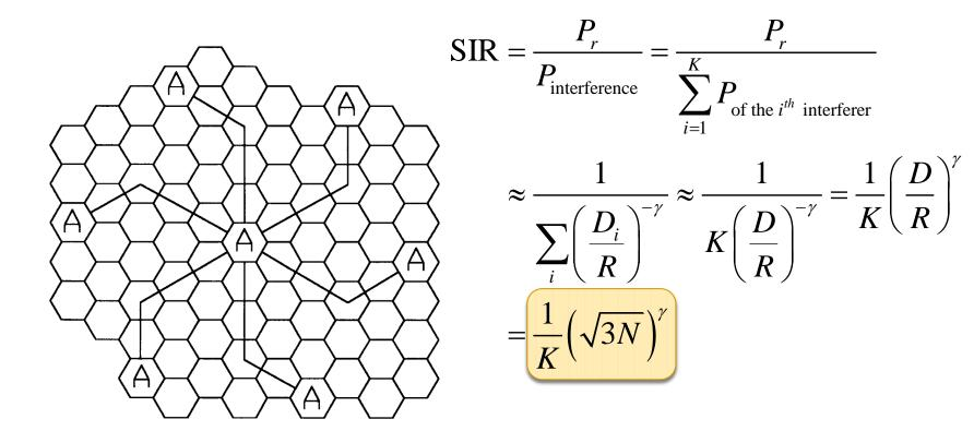
As the cell cluster size (N) increases, the spacing (D) between interfering cells increases, reducing the interference.
